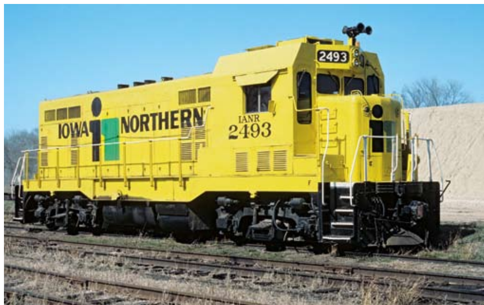
Above: On April 18, 1989, CF7 2493 rests between assignments at Bryant Yard in Waterloo. This unit began life in 1949 as Santa Fe F7A 300L. It entered Santa Fe’s CF7 rebuild program at the railroad’s Cleburne, Texas, shops in 1974, emerging as number 2493. During the 1970s, the CF7 program converted 233 aging F-series cab units into road switchers. Santa Fe went on to sell a number them to shortlines all across the country. The 2493 came to the IANR in 1987, retaining its Santa Fe road number. — John Leopard photo
